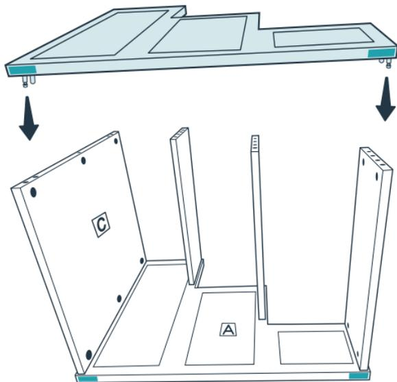
Connect the remaining side panel and secure the connections with cam nuts. Attach the self-adhesive feet to the four bottom corners and turn the steps upright.
