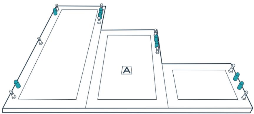
Insert wood dowels into the remaining holes in each side panel.
