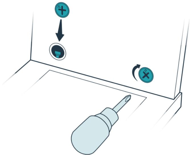
Insert cam nuts into the holes in each riser next to where the panels are connected. (The arrow on the cam nut should point toward the cam bolt.) Tighten the cam nuts to secure the connections.
