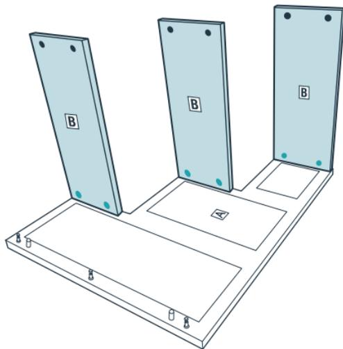
Connect the risers to one side panel with sides B facing inward.
