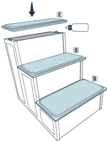
Squeeze glue into the slots on the top edge of the side panels and place a wood biscuit in each one. Starting at the top of the steps with tread E, attach each stair tread by applying glue to the slots on the underside of the tread, lining it up with the wood biscuits and pressing down.
