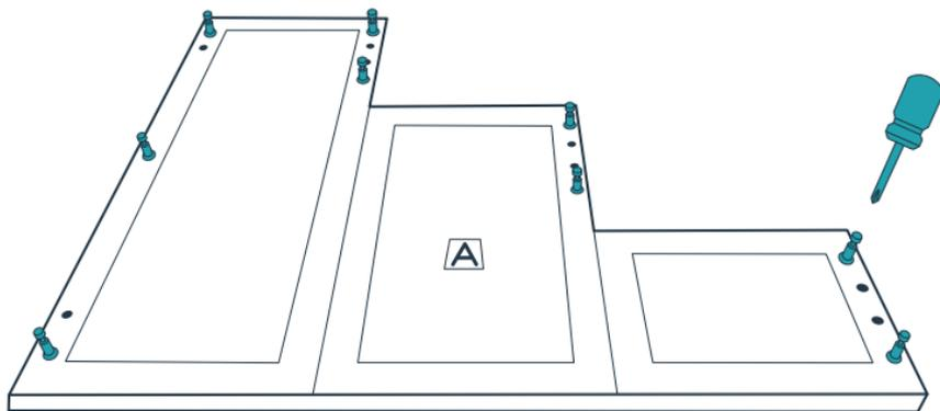
Lay both side panels flat with side A facing up. Screw cam bolts into the threaded holes in each side panel.
