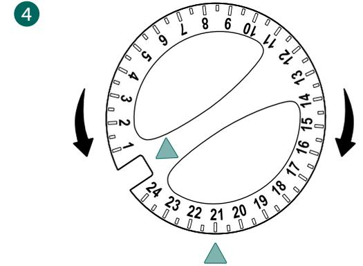
4 Set the feeder timers by turning each dial until the arrow on the feeder points to the number of hours between now and when you want your pet to be fed. (You can set it up to 24 hours in advance, in 1/2-hour increments.)
