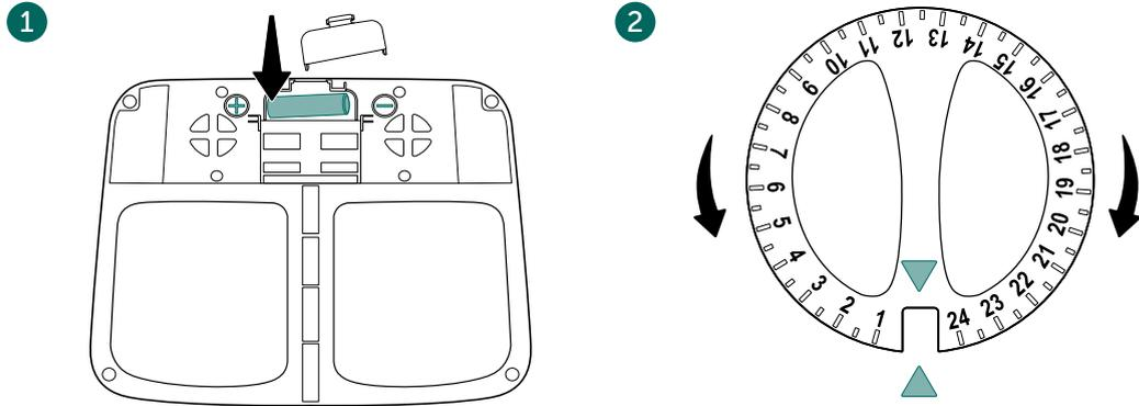
1 On the bottom of the feeder, remove the battery door and insert one AA alkaline battery. The battery compartment is very snug—it is easiest to insert the positive (+) end of the battery first, then press the negative (-) end into place.
