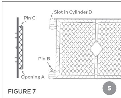
**STEP 5** Attach the mounting connector side B to panel 2 by setting opening A over Pin B, push down in order to slide Pin C into the slot of Cylinder D. See Figure 7.
