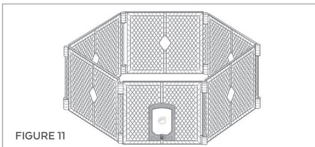
Begin setting up your enclosure by unsnapping the gray carrying strap and carefully unfolding the panels to form a hexagon. See Figure 11. When you have finished unfolding the panels, there will be two unconnected panels arranged as shown in Figure 12. Make certain that the pin in Cylinder B is up as shown. Begin connecting the panels together by gently lifting up on panel 2 and setting the Opening A (as shown in Figure 12) over Pin B located on panel 1.
