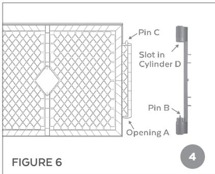
**STEP 4** Attach the mounting connector side A to panel 1 by setting opening A over Pin B, push down in order to slide Pin C into the slot of Cylinder D. See Figure 6.
