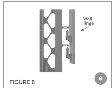
**STEP 6** Attach the mounting connectors, that are now attached to the panels, to the wall hinges by aligning the horseshoe shaped hoops on one side of the gate over the pins on the wall hinges to set the gate in place. See Figure 8. **NOTE:** Always lift up on the end panels to ensure that the gate is properly secured and locked in place.
