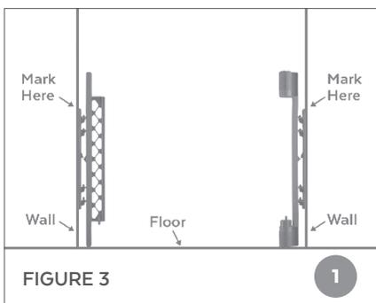
**STEP 1** Position both of the preassembled wall mounting connectors/wall hinges, vertically so the wall hinge pins are facing upwards on the wall, and the mounting connector is as close to the floor as possible. Mark the top of each wall hinge. See Figure 3.
