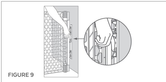
To remove the gate from the wall hinge, press on the locking boss located on the center of the wall hinge (See Figure 9), and lift the panel itself until the gate rib clears the locking boss.
