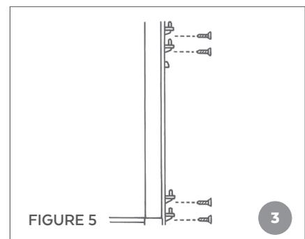
**STEP 3** To attach the wall hinge to the wall, align the top with the mark drawn in Step 1. Mark the top hole and pre-drill a 1/8" pilot hole. Attach the top of the wall hinge in place with a screw. Proceed down the hinge and install a screw into each screw hole with screws provided.
