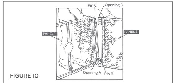
To disconnect two adjoining panels, select one of the joints where the panel pushes down (panel 1), as shown in Figure 10. Gently press down on panel 1 while lifting slightly on panel 2. This will enable you to slide Pin C free of Cylinder D (see Figure 10). Then lift up on panel 1 until Opening A (see Figure 10) is free of Pin B.
