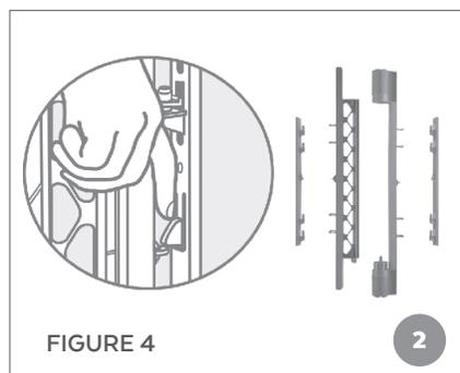
**STEP 2** Separate the mounting connectors from the wall hinges by pressing inward on the locking boss located in the center of the wall hinge. Lift up on the connectors to free them from the wall hinge. See Figure 4 for removal from wall hinge.
