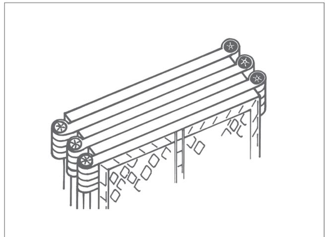
Your gate folds compactly for transport or storage. You must, however, fold the panels properly. Gently fold the panels (without jerking them or slamming them together) in alternating directions like an accordion.
