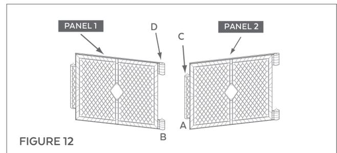
Now locate the slot on the lower end of Cylinder D. See Figure 12. This slot tapers to an opening that accommodates Pin C. Gently press down on panel 2 while aligning Pin C with the slot in Cylinder D. While maintaining downward pressure on panel 2, lift slightly on panel 1, and slide Pin C through the slot and into the opening as shown.
