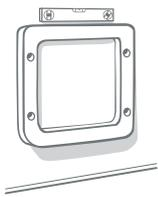
4 Stick the external frame to the wall on the inside of the house, lining up the pencil mark and bottom of the frame with the mark you have made on the wall. Use a spirit level to ensure that the frame is level.
