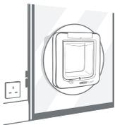
6 From the inside of the house, slide the tunnel of the main assembly through the hole in the glass.
