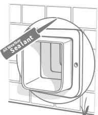
18 We recommend putting some waterproof sealant between the tunnel and the external frame to prevent water getting into the wall cavity.
