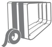
5 Apply superglue to the four tabs of the tunnel extender and fit the tunnel extenders together. When the glue has dried, apply weatherproof tape to the outside of the tunnel.
