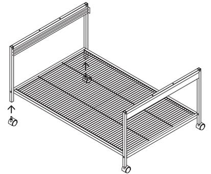
Flip assembled unit over and fully insert casters into frame legs.
