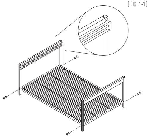
Attach the storage shelf to the leg frames to create the base. Back ends of leg frames have a backstop tab at the track ends (fig.1-1).
