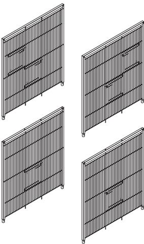
Stack the side panels in place on the base. For correct assembly, note these details:
