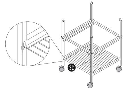
By leaving Step 2 screws loose, there should be a little play in the legs. Insert the U-shaped ends into the slots on the left side first; then insert the right side.
