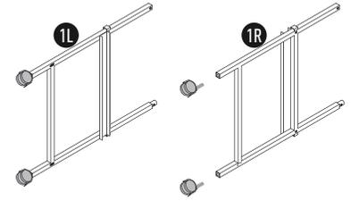
**2** The tray channels on the frames should be facing each other, and the rounded post ends (at the top back of the frames) should be closest to the floor. Locate the duplicate frame front (2F) and frame back (2B) bars and attach them to the side frames (just above the tray channels), with long hex screws. **DO NOT FULLY TIGHTEN.**
