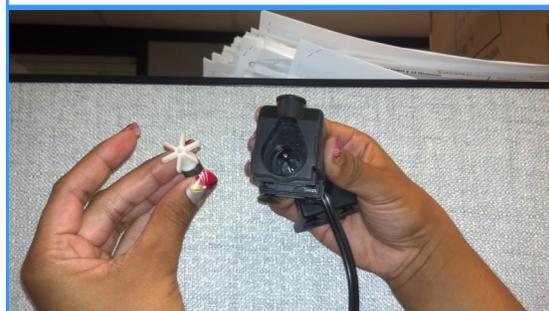
**After thoroughly cleaning, place all components back together and return to your pump to the filter / water environment before turning on.**
