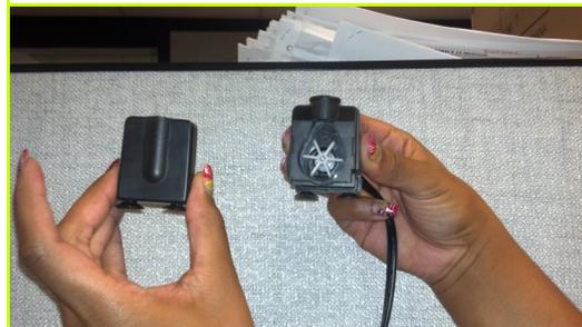
5. Remove the impeller gently—you will feel a slight tension as the magnet releases from the pump.
