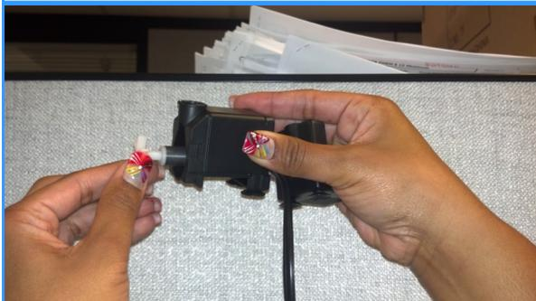
6. Clean the impeller and the "well" of the pump thoroughly.
