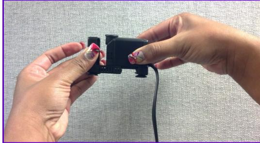
3. As seen below, the "ribbed/vented" piece of the bottom plate slides off as one piece with the front plate.
